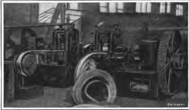
Fig. 17. Cold-rolling Strip Stock
